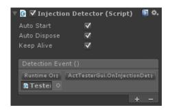
This detector has no additional options to tune except the common ones (note, when started from code, you pass callback which accepts string argument – detection cause).
