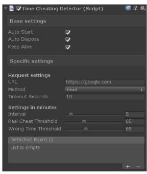
**URL:** absolute URL to the resource which will return correct Date response header value to the HEAD or GET request. When running in WebGL, URL automatically changed to the current domain if necessary, to avoid CORS limitations.
