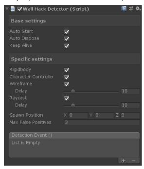
**Rigidbody:** enable this module to check for the "walk through the walls" kind of cheats made via Rigidbody hacks. Disable to save some resources if you're not using Rigidbody for characters.
